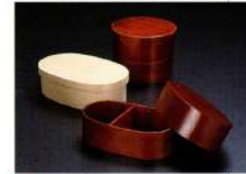
3 Magemono (Shioiri City) E-3 Soba and tea tools made from bending thin Kiso-Hinoki cypress boards.
